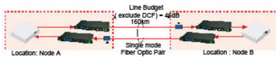
Figure A: MS1025 point to point application
